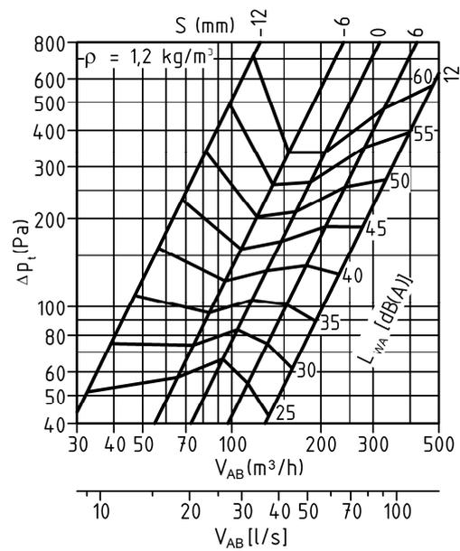
**Pressure loss and noise level (supply air)**
