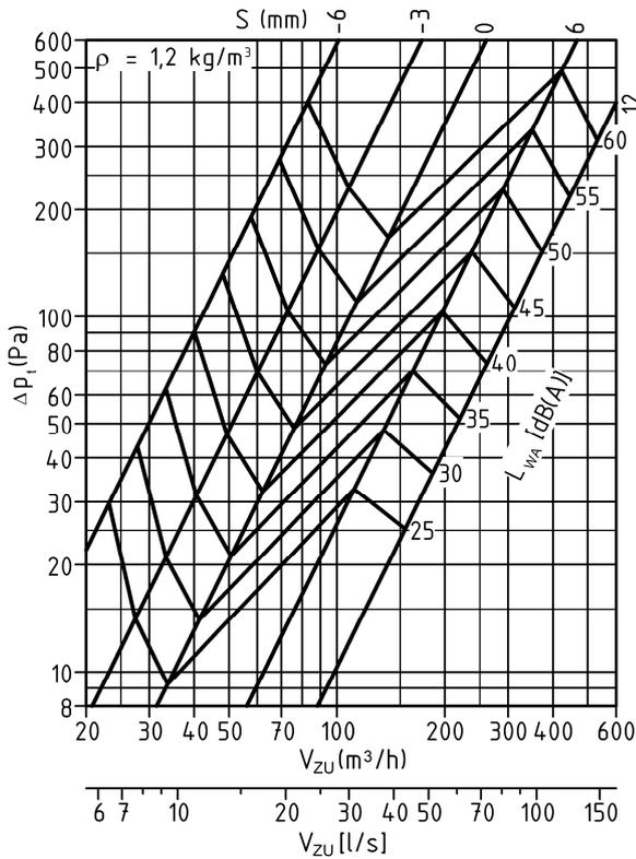
**Pressure loss and noise level (return air)**
