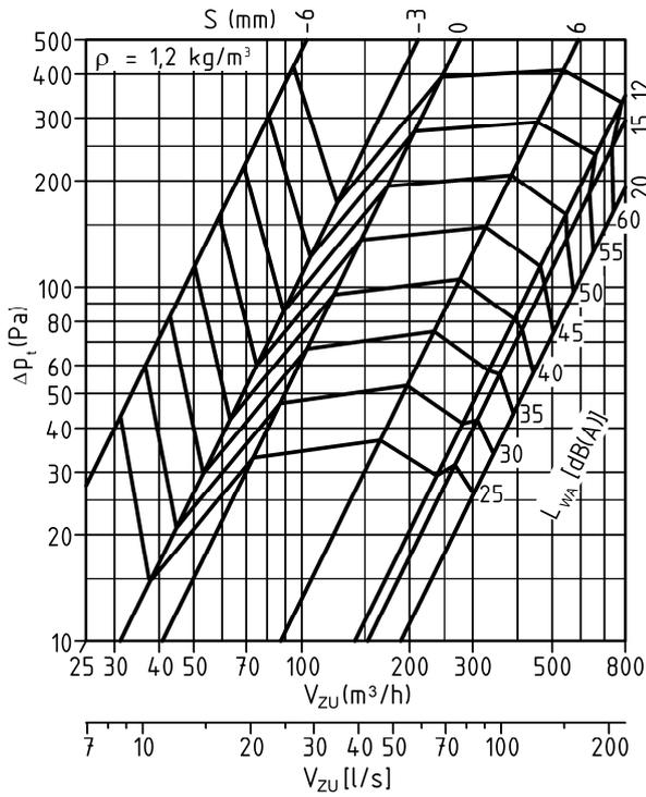
**Pressure loss and noise level (return air)**
