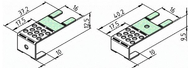
For models with screw mounting, 4 mounting brackets (mounting aids) are supplied loose.
