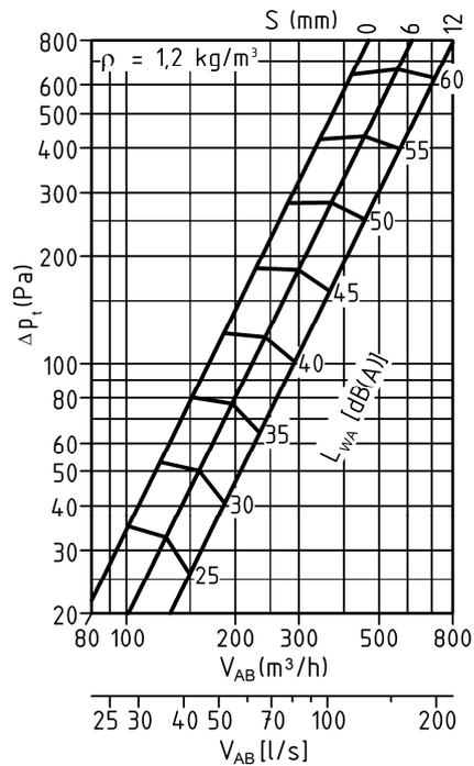
**Pressure loss and noise level (supply air)**
