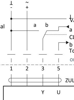
Connection of external switching contact (SMV)
