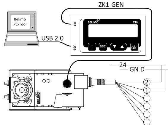
Local connection via service socket of the MF/MP using a ZK1-GEN cable.
