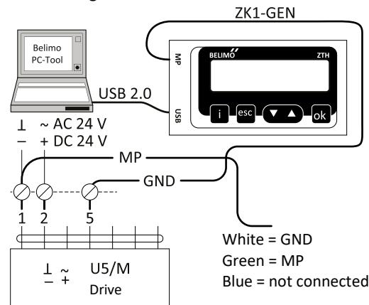
Local connection via connecting cable of the MF/MP using a ZK2-GEN cable.
