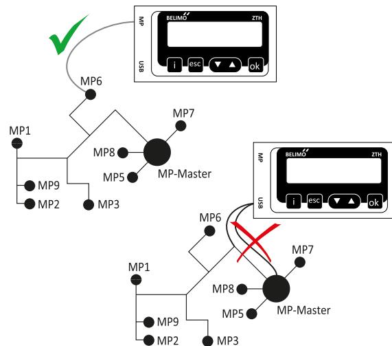
Restriction: Direct connection in an MP network or to an MP-Bus master is not possible.
