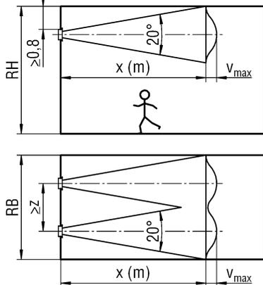
For the diagrams to be correct, the distance  $z$  between two grilles must be  $\geq x$  (m)  $\times 0,2$ .
