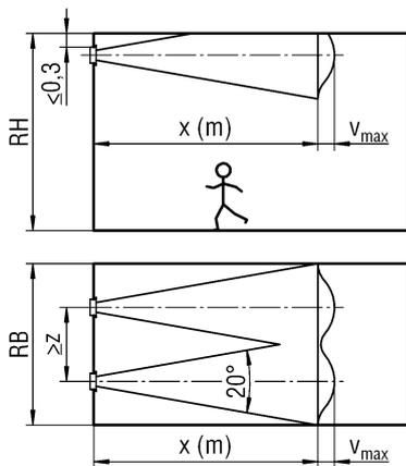
For the diagrams to be correct, the distance  $z$  between two grilles must be  $\geq x$  (m)  $\times 0,2$ .
