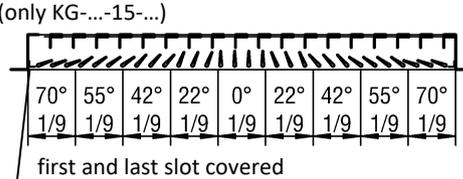
The angle of propagation of the air jet and thus the length of throw can be affected by adjusting the vertical air deflection blades.
