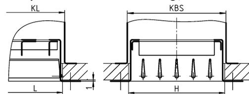
with plenum box below the ceiling / in front of the wall
