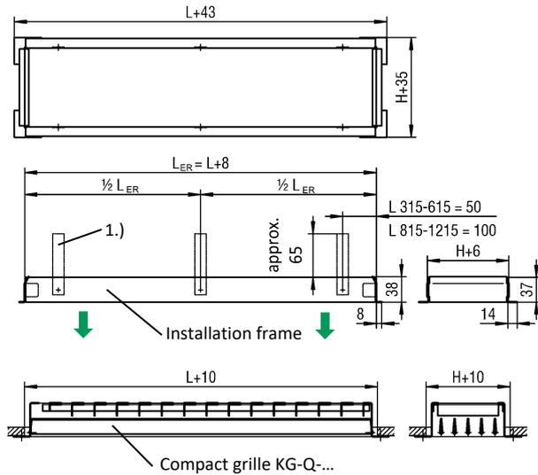
**Attention: Change of installation opening for installation with installation frame!**
