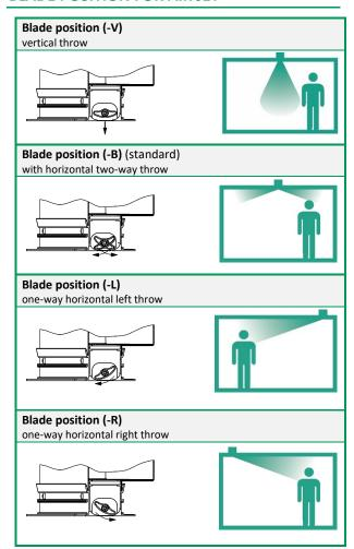
With blade positions (-L) and (-B), the concentric air throw toward the inside may result in greater velocities and turbulence.
