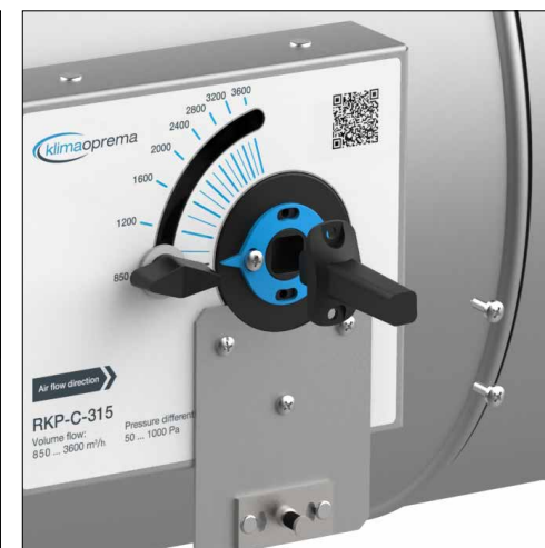
4. Install the motor shaft with two self-tapping screws 3,9x13 DIN 7981. (1,5 Nm)
