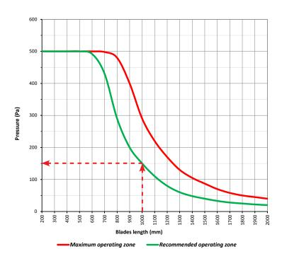
We recommend that the counter-pressure does not exceed 150Pa for a 1000-mm long AS damper.
